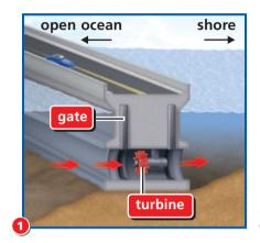
The dam's gates are open as the tide rises. Notice that the water level is the same on both sides.
