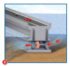
At low tide, the gates open and the water rushes out, spinning turbines that generate electricity.
