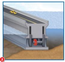
When the tide begins to lower, the gates close, trapping water behind the dam.
